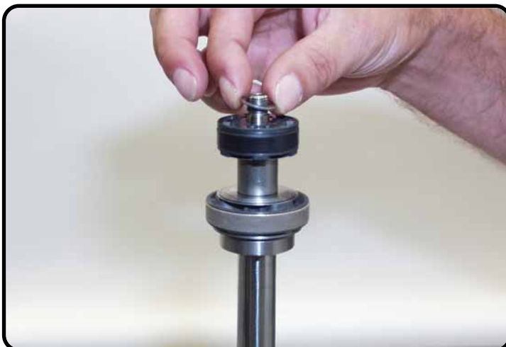
Assemble the ring of check-valve setting 2.
