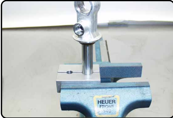
Clamp the piston rod in T1202S.
