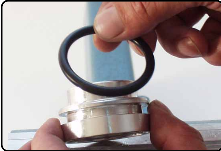
Remove the O-ring
