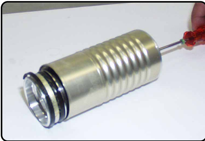
Pay attention to the assembling direction! Push with T170S the separation piston out of the reservoir.
