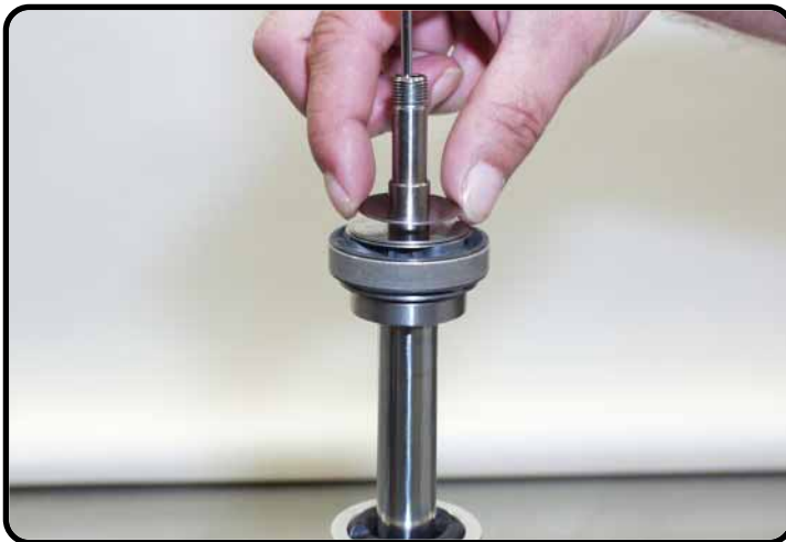
Assemble rebound setting 1.
