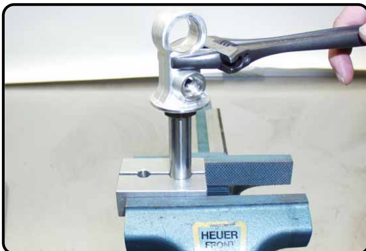
Unscrew the mounting-eye.
