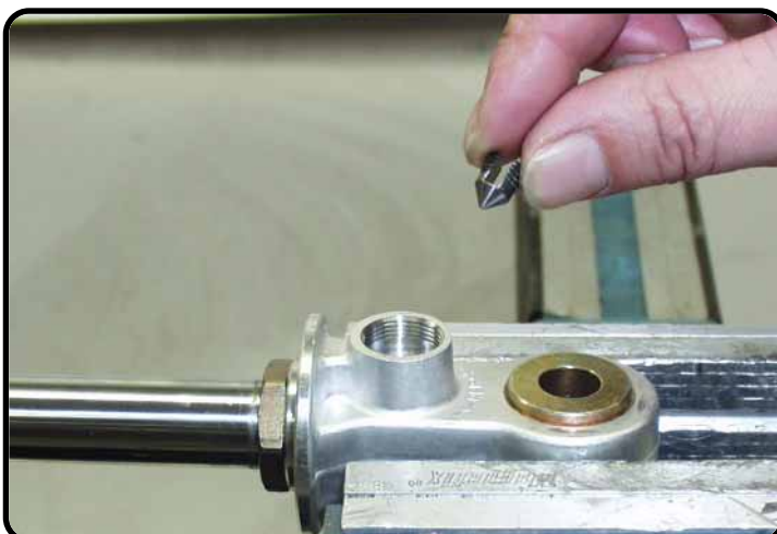
1. Replace the rebound adjustment needle.
