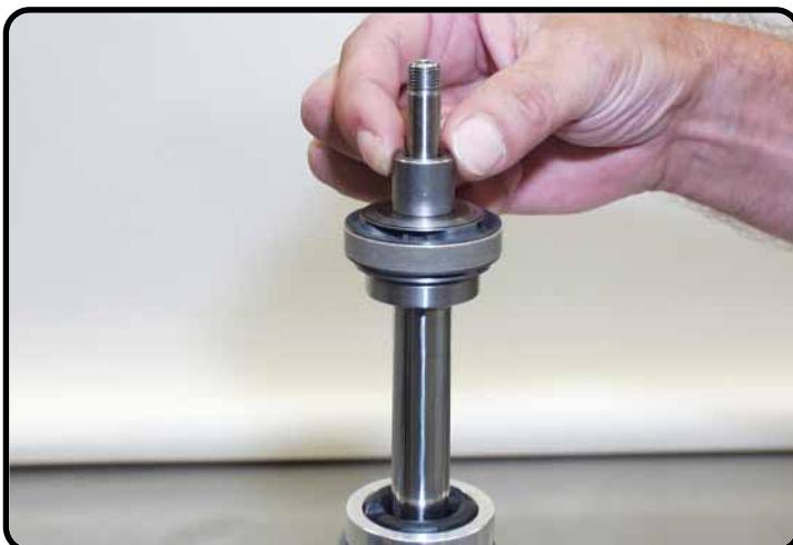
Replace the intermediate bush.
