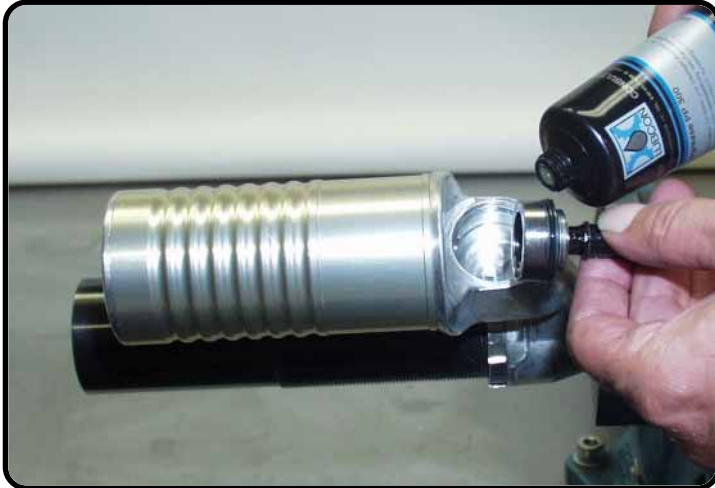
Grease the O-ring of the DCC piston.
