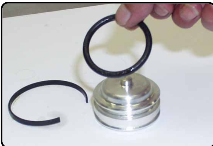
Remove the O-ring and piston ring.
